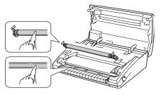
6. Replace the roller. Make sure the roller's tabs lock into place.
